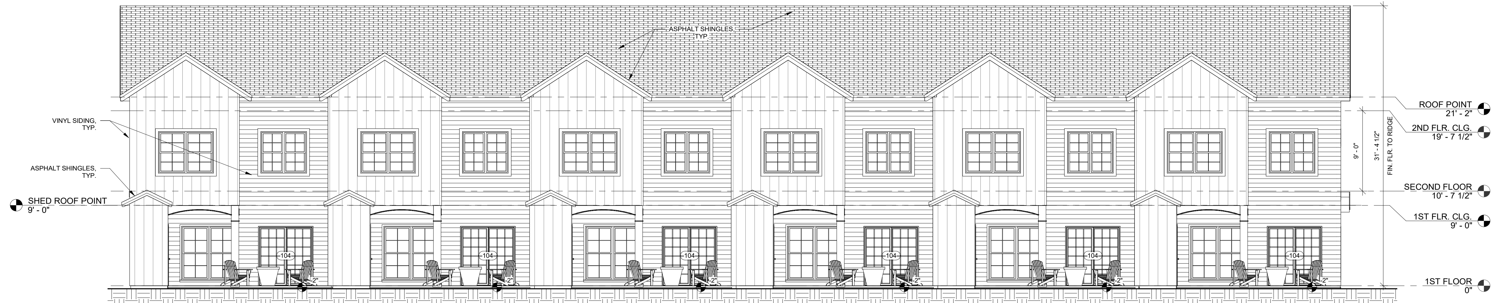
4 BLDG 1 & 2 TYPICAL REAR ELEVATION 3/16" = 1'-0"
