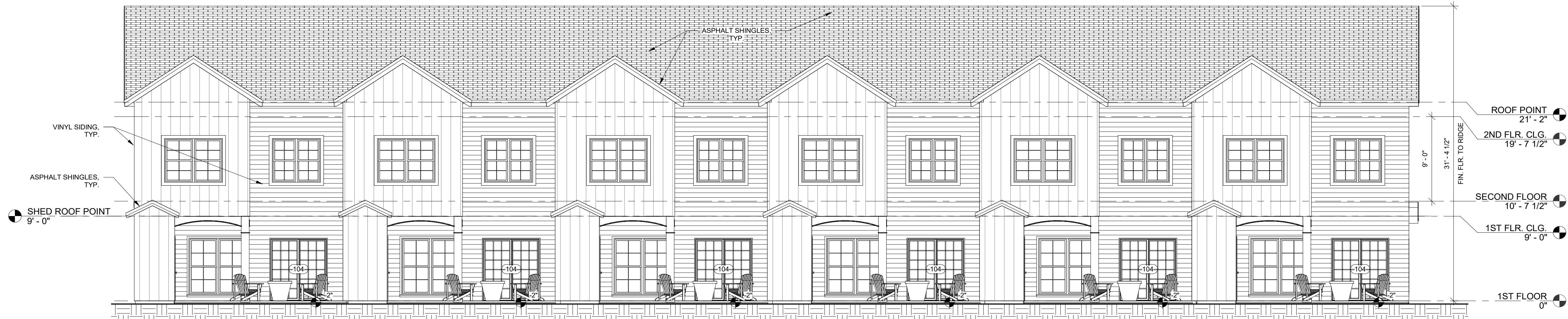
4 BLDG 1 & 2 TYPICAL REAR ELEVATION 3/16" = 1'-0"
