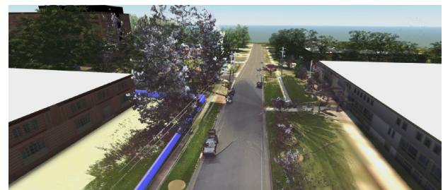
Pictured above is a full 3D model that allows clash detection, virtual walk-throughs and 3D mockups.
