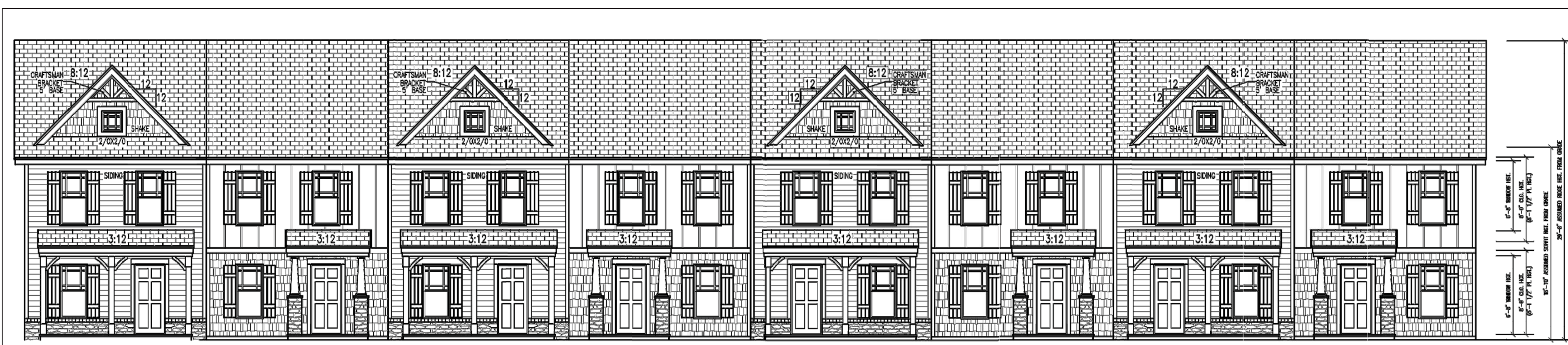
FRONT ELEVATION (8 UNITS) NOT TO SCALE *ALL UNITS ARE 2 BEDROOMS/ 2 BATHS EXTERIOR MATERIALS: VINYL SIDING, STONE, AND ASPHALT SHINGLES
