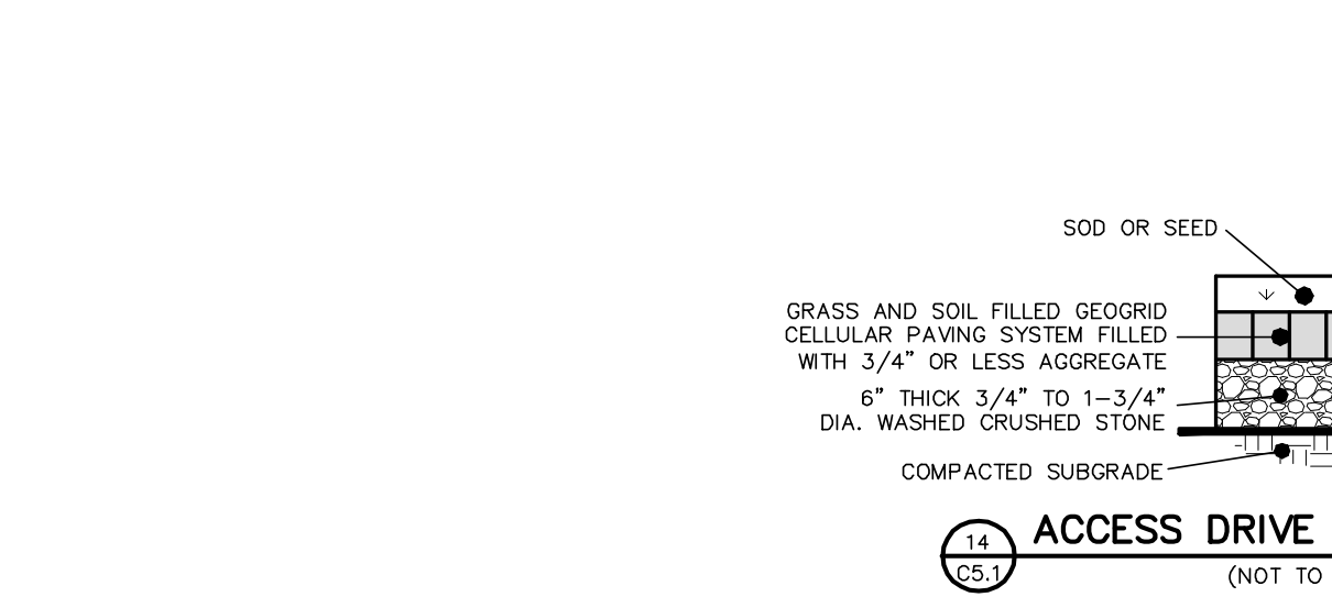
14 ACCESS DRIVE GEOGRID SYSTEM (NOT TO SCALE)
