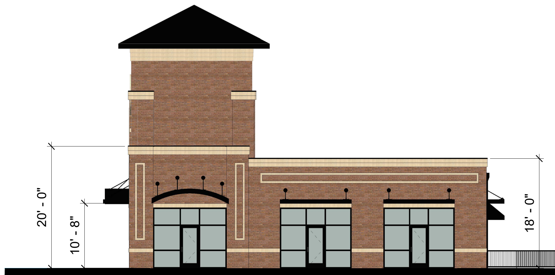
③ EAST ELEVATION - BUILDING A 1/8" = 1'-0"
