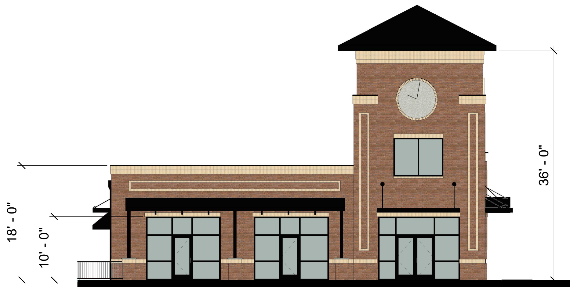
② WEST ELEVATION - BUILDING A 1/8" = 1'-0"
