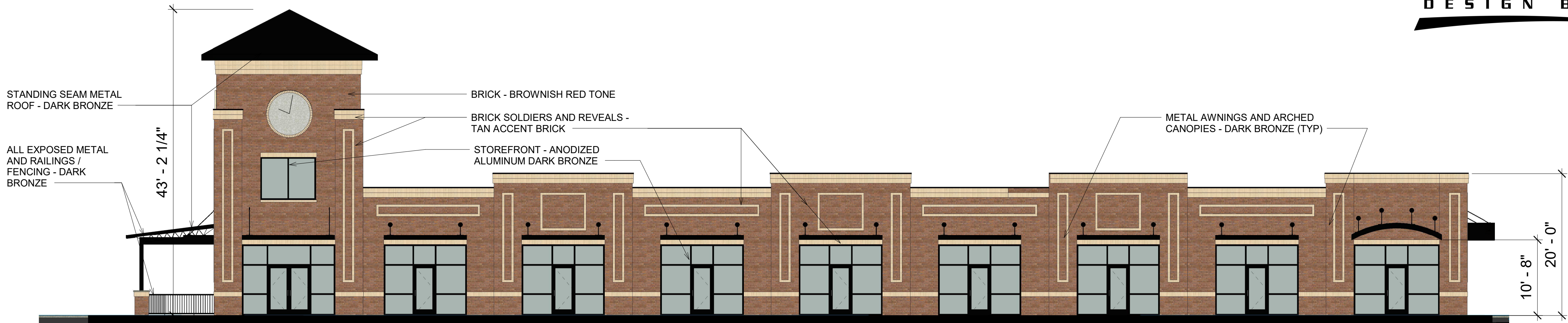
① SOUTH ELEVATION (MAIN STREET) - BUILDING A 1/8" = 1'-0"
